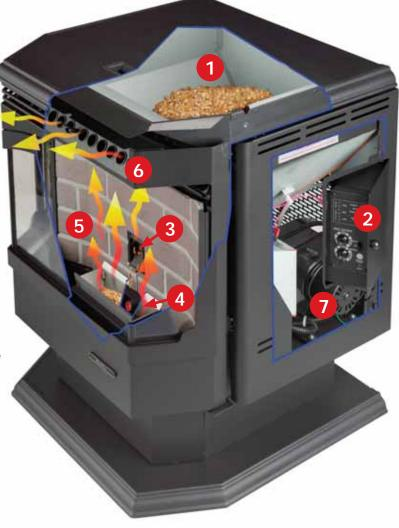
7. A super-quiet variable speed convection fan (130 CFM on compact and 165 CFM on large models) draws in the cool room air and pulls it around the heat exchange system. This transfers the heat from the appliance and delivers hot air directly into your home.
